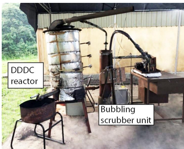
Figure 2. The DDDC reactor during the field operations at Meewathura farm premises
